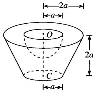
Mortar  $S$  is placed on a rough horizontal plane with its lower circular face touching the plane. Now, the plane is tilted upwards slowly. The coefficient of friction between the mortar and the plane is 0.9. Show that if  $\alpha < \tan^{-1}(0.9)$ , then the mortar stays in equilibrium, where  $\alpha$  is the inclination of the plane to the horizontal.
